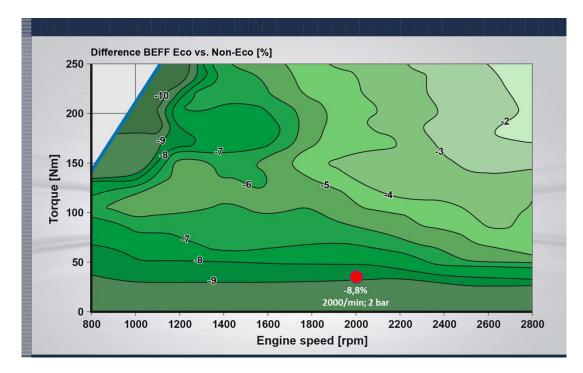
Fig. 12: Consumption map – differences between basic engine and Eco
