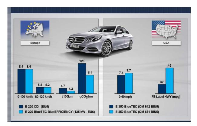
Fig. 13: Performance/consumption of OM 651 Eco in comparison with predecessor
