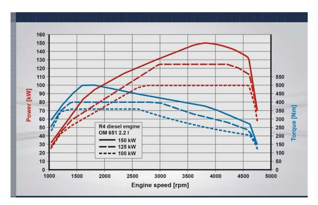
Fig. 5: Output and torque curves for main OM 651 variants
