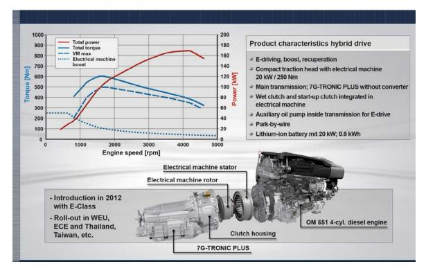
Fig. 10: Use of the OM 651 in hybrid applications
