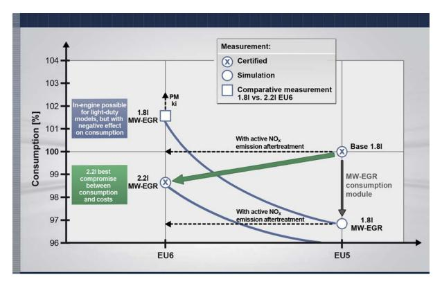
Fig. 8: Development options for the EU6 OM 651 in the trade-off with emissions requirements
