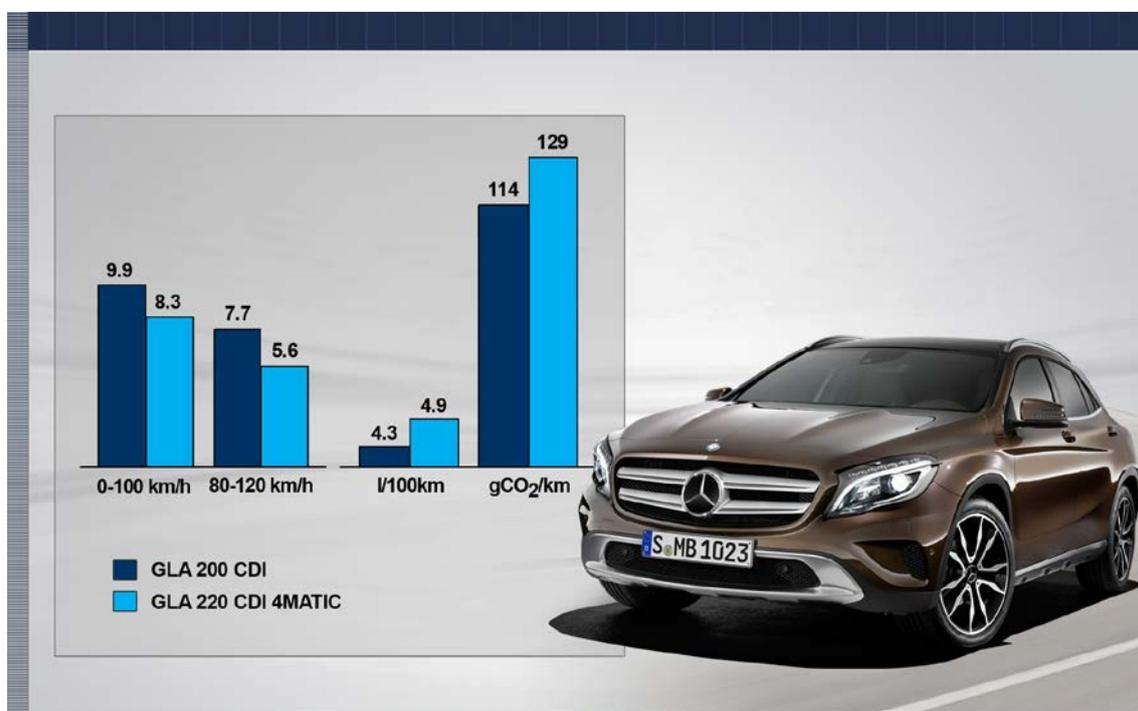
Fig. 14: Performance and consumption of OM 651 Eco in the new GLA200/220 CDI
