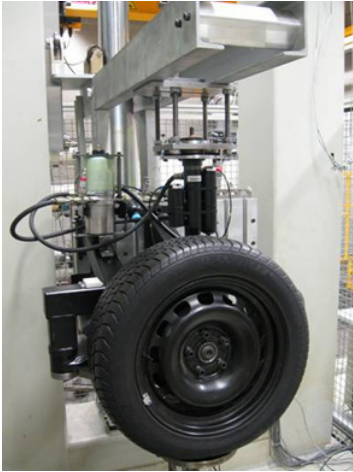
Picture 1: quarter car test rig overview
