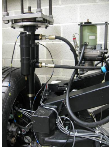
Picture 2: quarter car test rig with ACOCAR suspension
